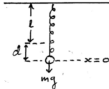
When mass  $M$  is attached the ensuing motion is SHM and the equation of motion is
